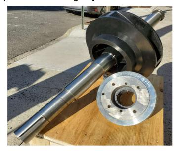
A 24" Diameter SIMSITE® Structural Composite Carbon Fiber Impeller on a type 316 Stainless Steel Shaft with a SIMSITE® Stabilizing Bushing pressed into the sealing chamber.
