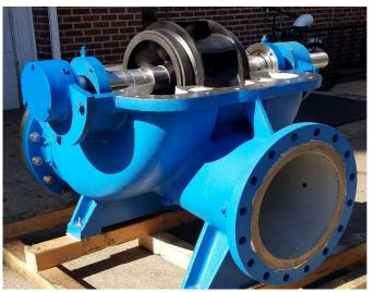
SIMS manufactures PUMP SIMSITE® structural graphite composite computer engineered and generated pumps and pump parts which are 100% machined on 5 to 8 axis robotic machining centers. SIMS uses state-of-the-art CFD techniques to engineer the vane geometries to maximize efficiency and performance specifically for the Customer's System. SIMS manufacture obsolete parts any centrifugal pump with quick deliveries.
